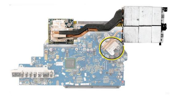
9. This shows the tamper-proof label on the top side of the logic board.
